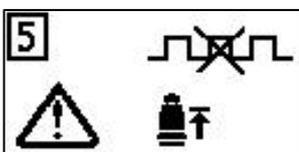
**Possible reasons:** The motor wire is disconnected, and the motor encoder wire is disconnected.
