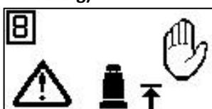
**Possible reasons:** The motor is blocked by an obstacle, the seat is locked, or the motor is short-circuited, or the encoder is wrong.
